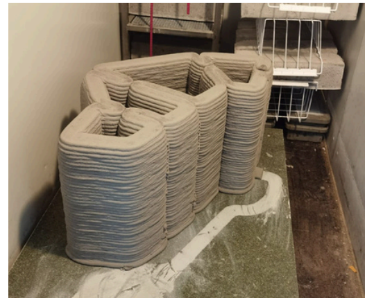
MINERALIZATION OF BLOCK IN CARBONATION CHAMBER
